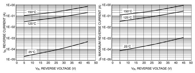
**Figure 3. Typical Reverse Current**
