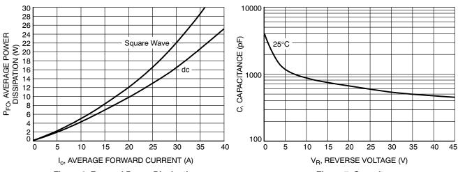
Figure 6. Forward Power Dissipation
