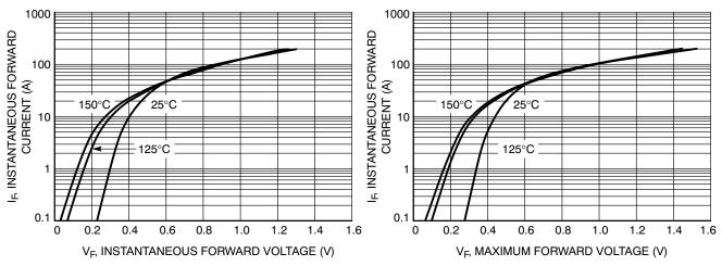
Figure 1. Typical Forward Voltage
