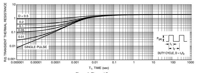
Figure 8. Thermal Response Junction-to-Case for MBR40L45CTG
